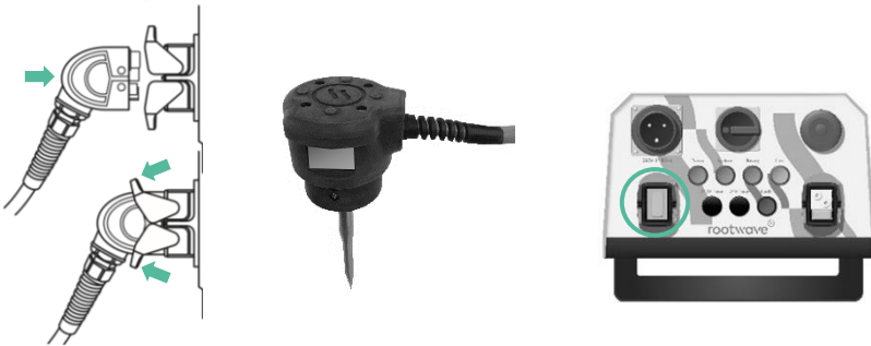
Figure 13 Connect the Safety Earth to the Power Module
